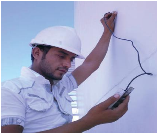
Test of coating in Tank
